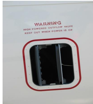
Pressure outflow valves
