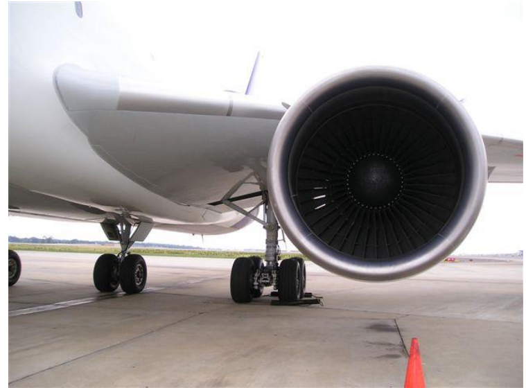
ENGINE INLET & LANDING GEAR
